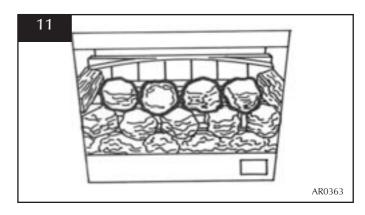
• Put the last three round coals behind the centre row and touching the back panel, Diagram 12
